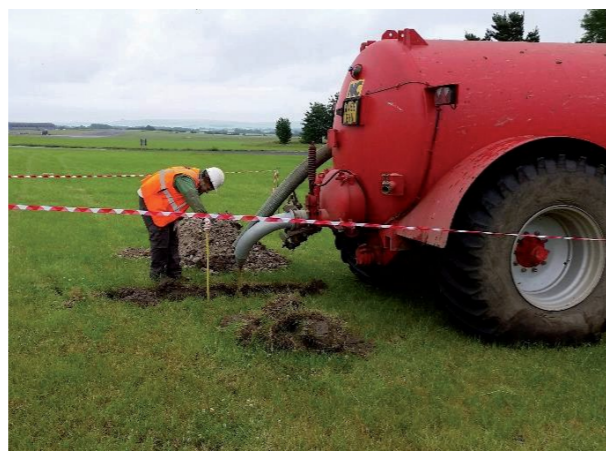
METHOD USED FOR SOAKAWAY TESTING 10,000 LITRE BOWSER RAPIDLY DIS- CHARGED INTO TRAIL PITS AND REPEAT- ED THREE TIMES
